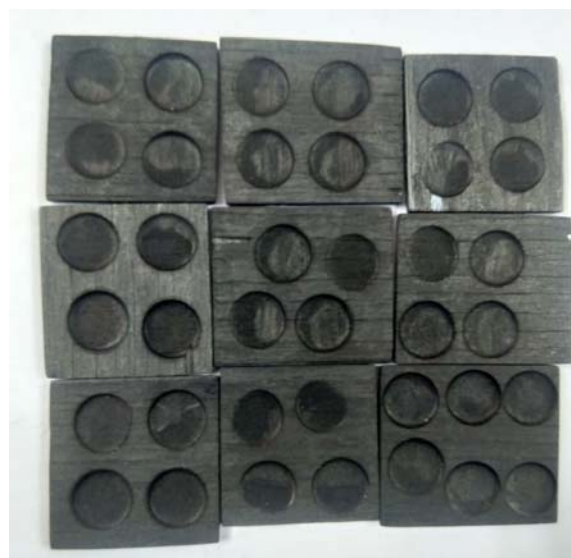
Figure 3: Holes of 8mm dia. machined on C/C composites
