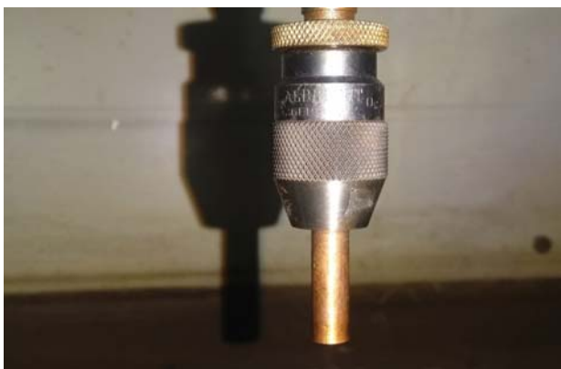
Figure 2: Keyless Drill chuck with copper tool ø8mm
